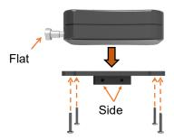
5.4 Install force gauge assembly onto the automated tool tester carriage ensuring side holes are aligned. Use QTY 2 M4-20mm Hex Socket Head Screws to secure as shown:
