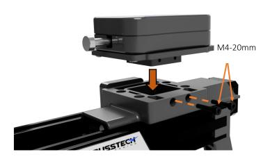
5.5 Loosen T-Nuts on RTTL0002 Tool Mount and slide onto automated tool tester from the left side ensuring T-Nuts are aligned properly in channels. Position on the left side of the rail and tighten T-Nuts by lifting the blue spring-loaded thumb screws and using a 2mm hex key to tighten the screws.
